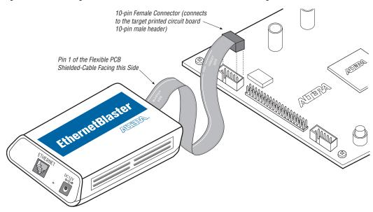
Figure 1–3. Connecting the EthernetBlaster Communications Cable to the Target Circuit Board
